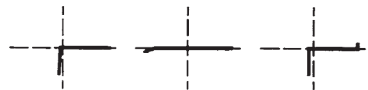
Typ: Normale Diode, Hochspann.-Diode, Z-Diode 12V Pole: Kathode-Anode, Kathode-Anode, Kathode-Anode Anschlüsse: (CT-Masse), (CT-Masse), (CT-Masse)
